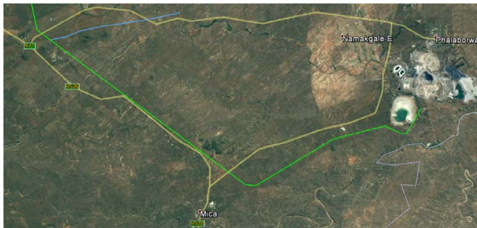
Figure 31: The last sector of Alternative 2 following the R526, crossing the R530 and then swings east to the Foskor substation.
